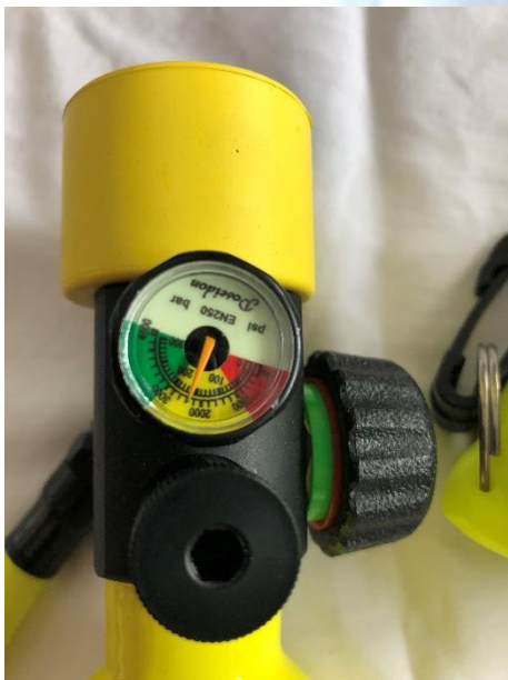
Pressure Gauge, Filling Connection & On/Off Green "ON" Red "OFF" indicator
