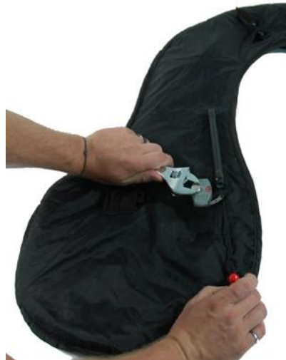
Figure 24I Step c. Mounting the Inflator Assembly
