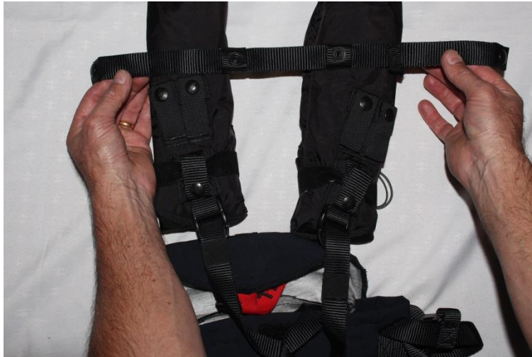
Figure 28ab Step i. The Chest Restraint Strap
