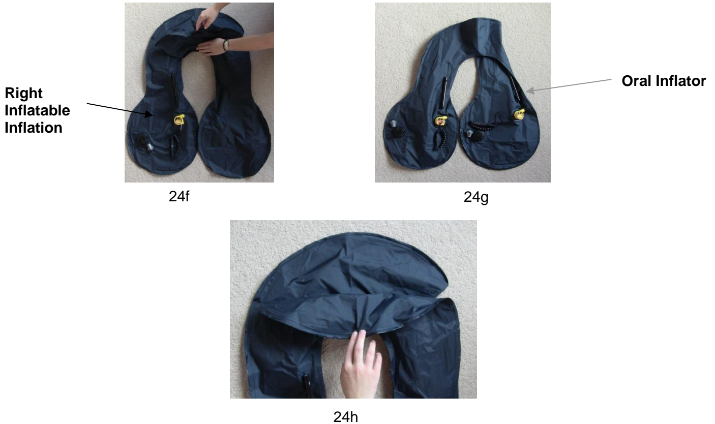
Figure 24f – 24h Step d. Layout of the Three Quarter-Inflation Cell Shapes
