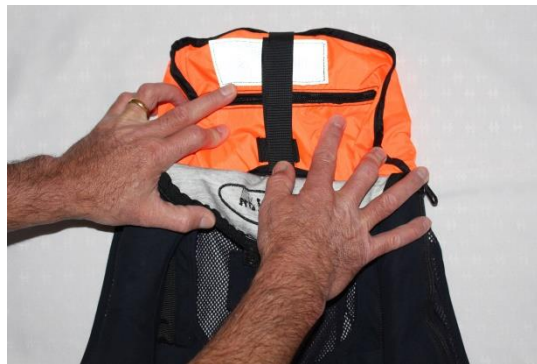
Figure 26w Step t Zipper Closure, Neck Area
