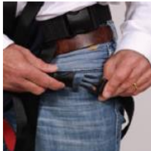
Figure 34l. Leg Strap Placement Around Legs
