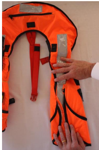
Figure 28m Step s. Packing Fold 9 Left Lobe
