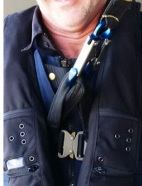
Figure 7c Lifting Harness Attachment Points
