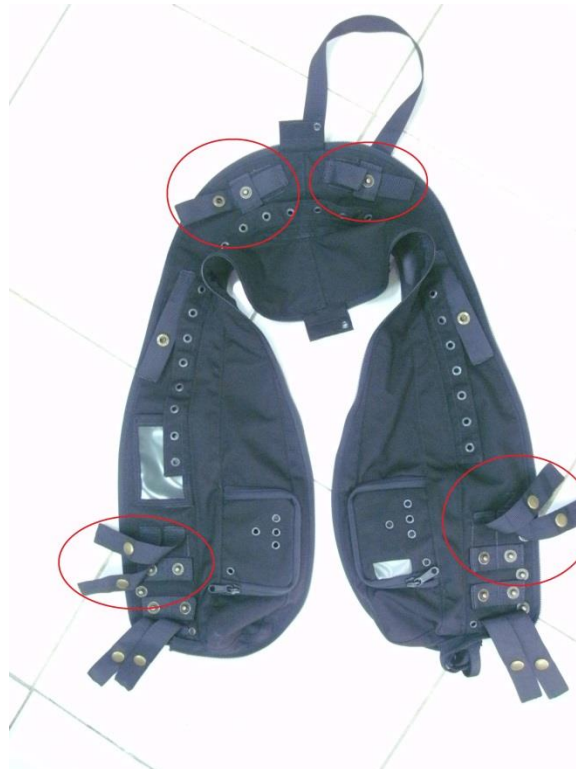
Figure 4b Webbing Attachments (Full Torso Harness)
