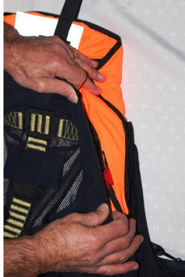
Figure 26v Step s. Zipper Closure, Right Lobe
