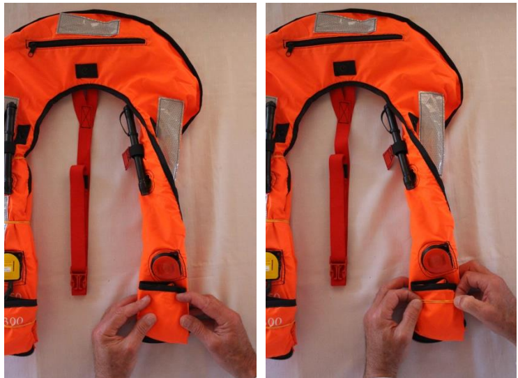
Figure 28o Step u. Packing Fold 10 Folding the base of the Lobe
