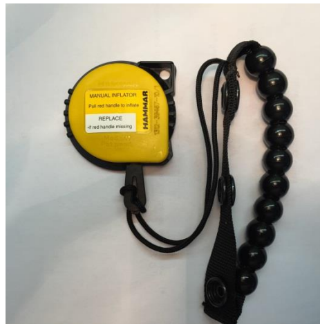
Figure 22i Step f. Re-Arming – New Manual Cap
