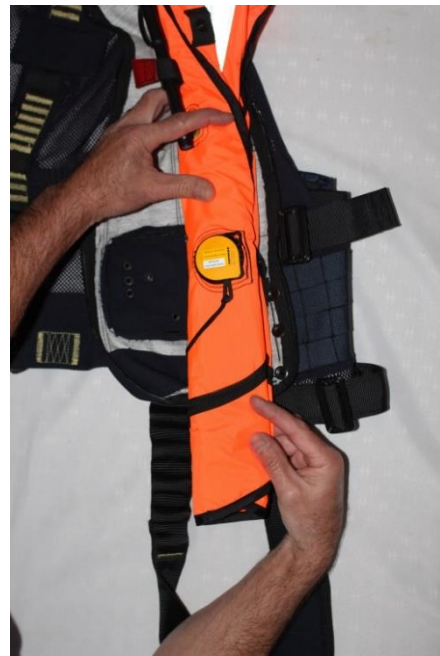
Figure 26s Step p. Packing Fold 9 – Actuator Upright
