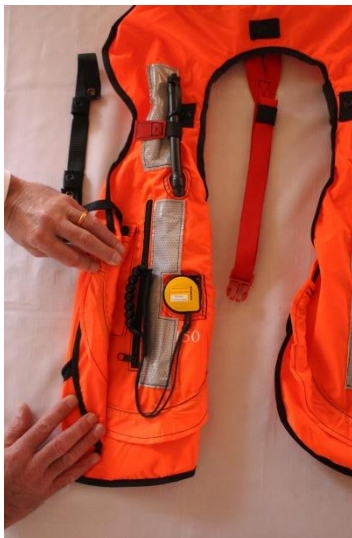
Figure 28f Step l. Packing Folds 3 and 4 Right Lobe
