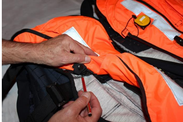
Figure 14f Step d. Webbing and Snap Attachment System at the Lobes
