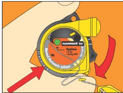
Figure 20k Step h. Re-Arming
