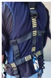
Figure 7b D Rings Fall Arrest and Restraint Attachment Points
