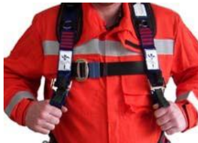
Figure 33k Step c Shoulder Straps - Pulling on the Webbing Tag
