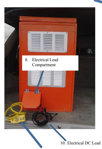
9. Electrical AC Lead with RCD Protector
