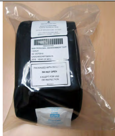
34. Insert desiccant packet into poly bag. Desiccant label, Manufacture date label, Expiration date label are placed on the poly bag. Heat seal poly bag closed.
