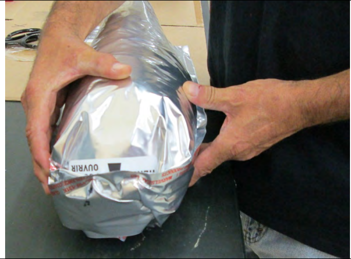
8. Fold the flaps down at the closed end of the bag as shown to avoid tearing while in the packing machine.
