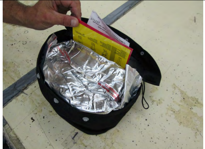
30. Place the donning card and lanyard into the pouch behind the suit along the curve.
