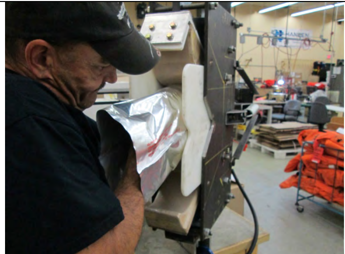
10. Push suit into the packer, keeping the side seams centered at both sides. Push into the packer as possible.
