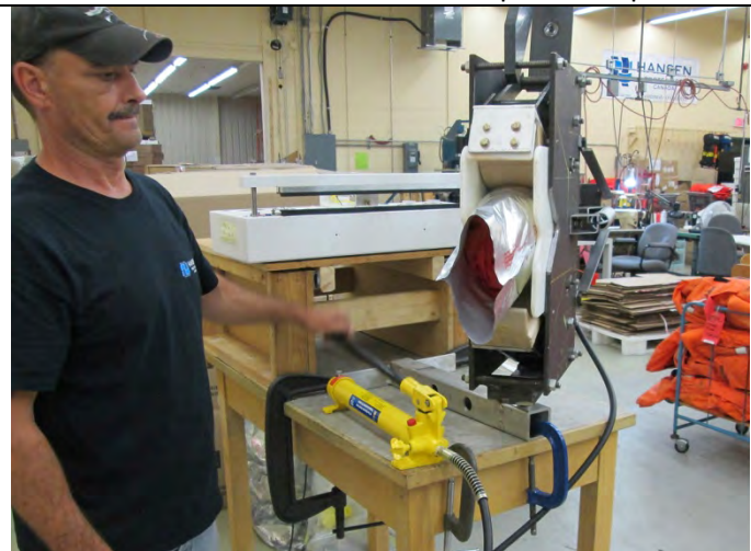
12. Pumping the handle will close the packer. Ensure
