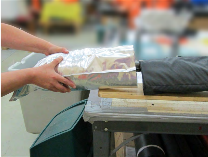
7. Remove the foil bag from the board when the suit has been pushed in as far as it will go.
