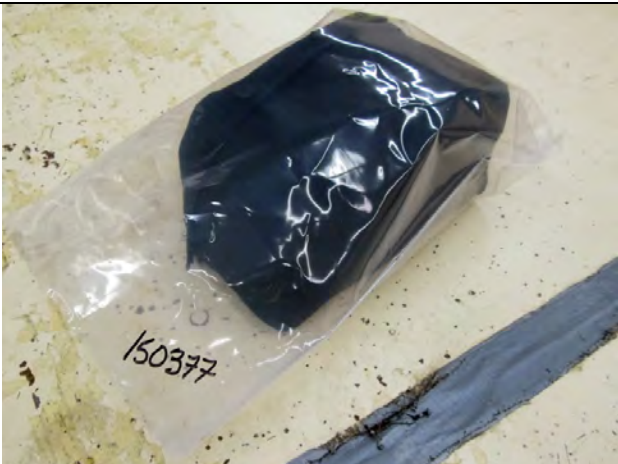
33. Insert in to poly bag with serial number neatly printed on the bag with permanent marker.
