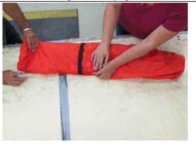
20. Roll the suit, starting at the feet. Roll keeping the edges tucked in at the sides. Proceed to packing into foil bag
