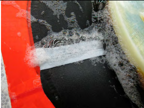
This image shows the side seam on the neck gasket leaking. Streaming bubbles
