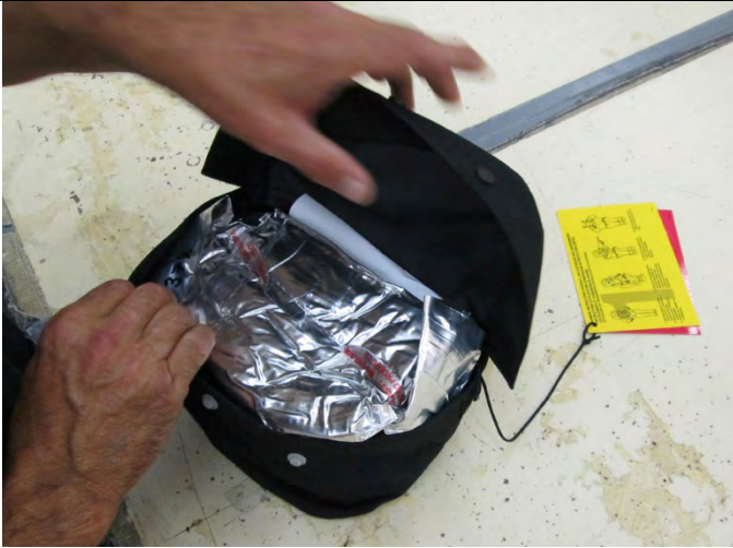
29. Insert into Nomex pouch with the curve at the back. Make sure the suit is evenly positioned in the pouch.
