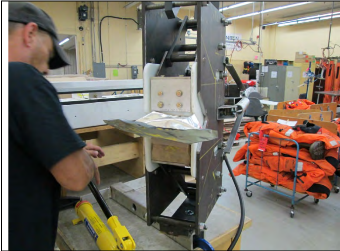
17. Straighten the bag opening so that it is extended away from the packer and both top and bottom parts are flat.
