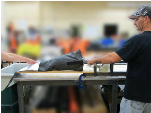
5. Turn the crank handle to push the suit down the sleeve and into the foil bag.
