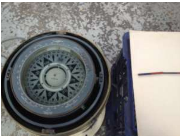
14, 15: Closing deflection test, -10 degrees.
