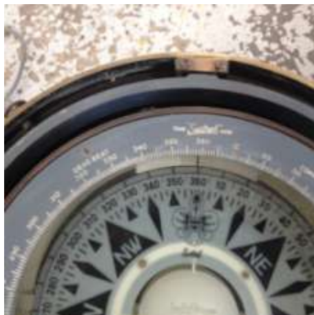
5: Return to 360 after deflection.
