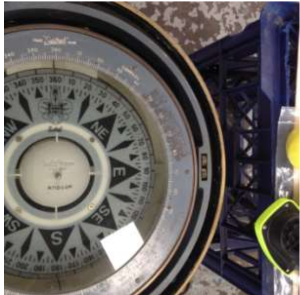
6, 7: First bottle test, 9393 unit, nil deflection.
